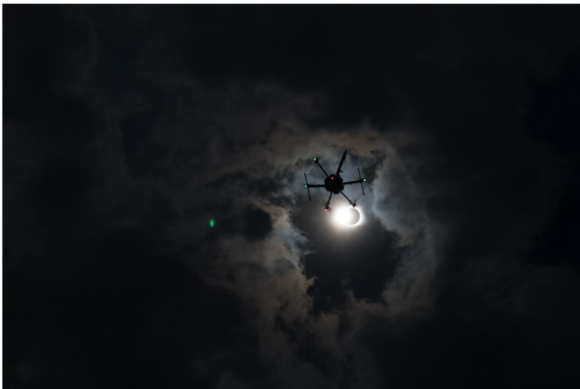
Figure A.5: Multirotor in-flight collecting TH data seconds before the total solar eclipse.
