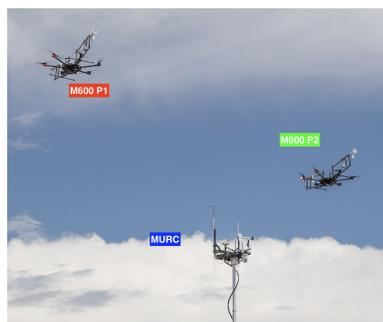
(a) Ten minutes of hover flight calibration of the UASs (M600P<sub>1</sub> and M600P<sub>2</sub>) with MURC (Mobile UAS Research Collaboratory).
