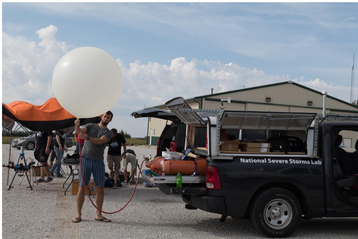
Figure A.6: Launching of Radiosonde Balloon For TH data observations
